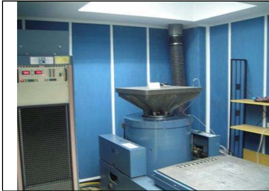
7. Vibration Test: Z axis
